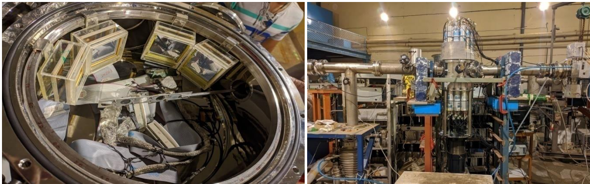
Experimental Setup, i) Charged particle detectors (Si-strips), ii) \gamma detectors, BGO, total 38
