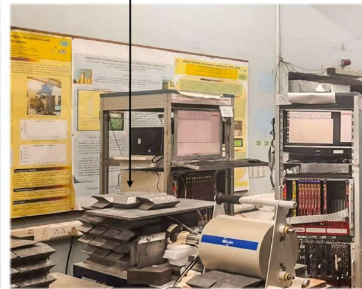
(c) Low background Offline \gamma - counting setup
