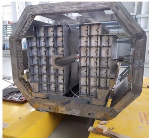
FHCAL assembled on the platform, modules are equipped with FEE and tested
