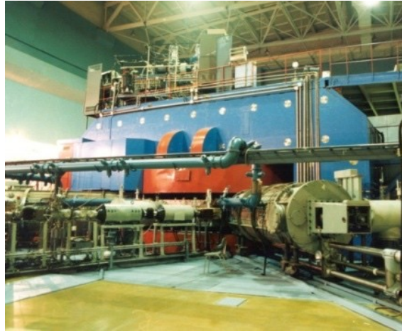
U-400M cyclotron: heavy ions 50 MeV/u (Li-Ne)
