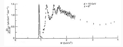
Data from SLAC, where the elastic peak at W = M has been reduced by a factor 8.5. [taken from Halzen, Martin, Quarks and Leptons]
